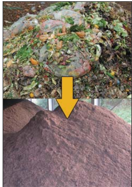
San Jose, Calif.'s waste-to-energy process starts with organic garbage (top) and ends with high-grade compost (bottom), and in between, it generates a considerable amount of methane for energy uses. Photo courtesy of Zero Waste Energy Development Co.
