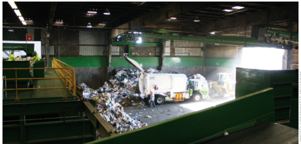
TRASH TALK: A truck dumps its load at the MSW tipping floor at GreenWaste’s dirty materials recovery facility.
